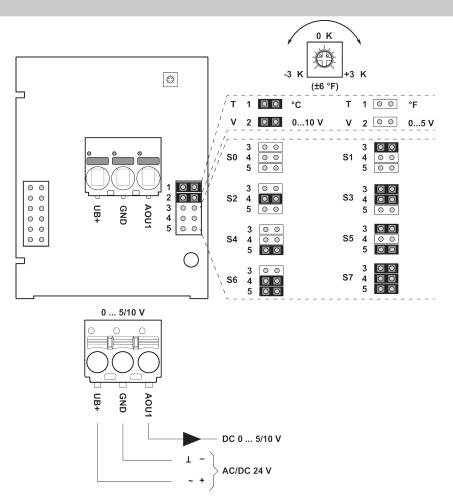
The adjustment of the measuring ranges is made by changing the bonding jumpers. The output value in the new measuring range is available after 2 seconds.
