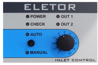
**POWER indicator light** – indicates the presence of power supply and charging the storage batteries.
