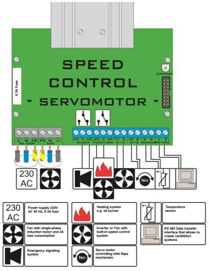
**Connector labelled as AC 230V** should be connected to the power supply (switching station). Using the circuit breaker 1P-B6 and overvoltage limiters of T1 and T2 type is obligatory. It is worth grouping the controllers on different phases (L1,L2,L3) while connecting multiple devices, in order to equally load the power line.
