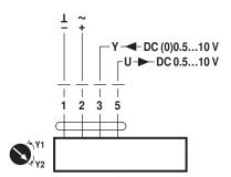
Override control (frost protection circuit)
