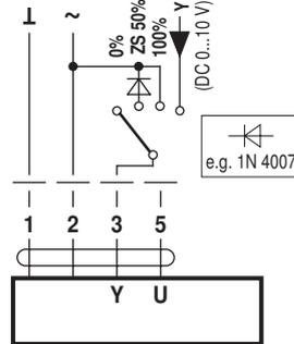
Control remotely 0...100% with positioner SG..
