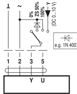
Control remotely 0...100% with positioner SG..
