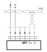
Signal assignment KNX: D+ = KNX+ (pink > red) D- = KNX- (grey > black) The connection to the KNX line should take place via WAGO connecting terminals 222/221.
