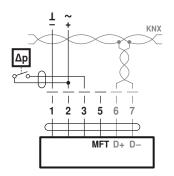
Requirements switching contact: The switching contact must be able to accurately switch a current of 16 mA@24 V.
