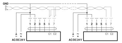
Connection with passive sensor, e.g. Pt1000, Ni1000, NTC
