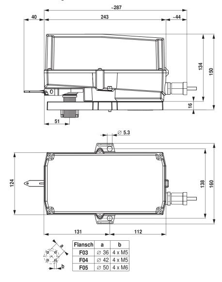
Rotary actuator (Retrofit), IP66/67, Open/close, 3-point, AC 230 V, 20 Nm  $\,$
