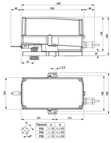
Rotary actuator (Retrofit), IP66/67, Open/close, 3-point, AC/DC 24 V, 20 Nm  $\,$
